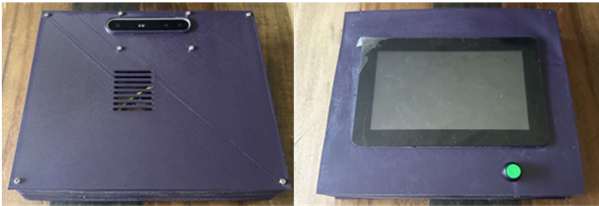
Fig. 24. Back (left) and front (right) faces of the Wireless 3D Scanning Device.
